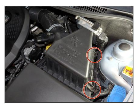
Unscrew the two phillips head screws. Use the reversible screwdriver that came with the car.
