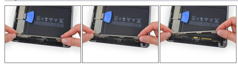
• Slowly peel the upper component cable bracket up out of the iPad—leaving the tape pieces on the bracket to make it easier to reinstall.
