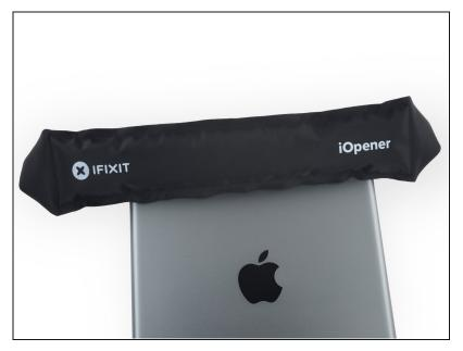
Lay a warm iOpener over the upper edge of the iPad and let it sit for a couple minutes to soften the adhesive holding the logic board in place.
