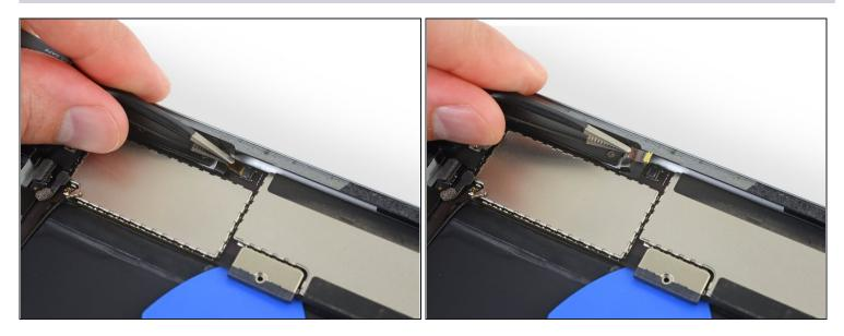
• Use tweezers to carefully pull the upper button assembly ribbon cable straight out of its connector.
