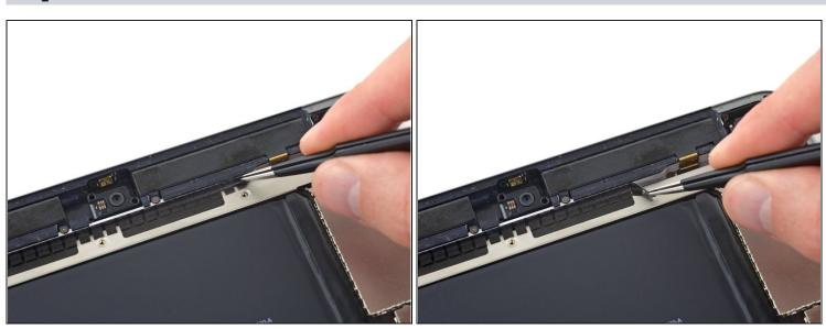
Use tweezers to start peeling back the tape securing the upper component cable bracket.
