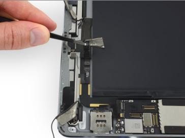
• Peel the tape toward the home button to uncover the speaker cable connector.
