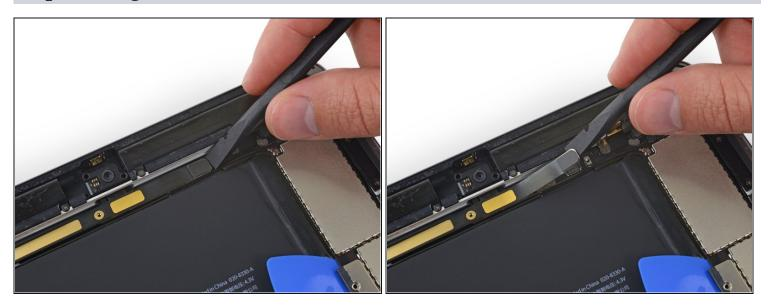
The following steps involve disconnecting many press connectors from their sockets on the logic board. When disconnecting these cables, be sure to pry up only on the connector, and not the socket itself.
