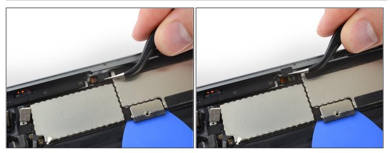
• Remove the piece of black tape covering the upper button assembly cable connector.
