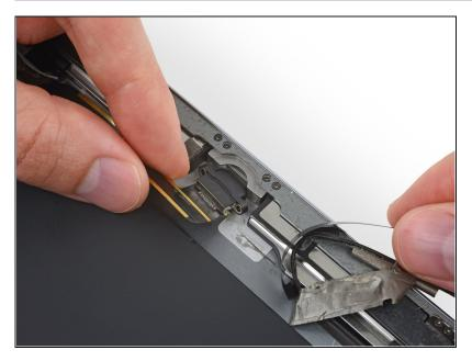
Pull the Lightning connector straight out of its recess in the rear case.
