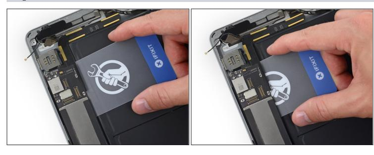
• Insert a plastic card underneath the lower end of the logic board, directly underneath the display connectors and Wi-Fi module.
