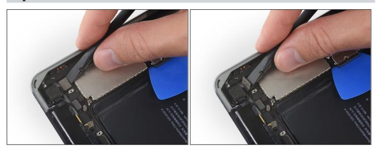
Use the flat tip of a spudger to disconnect the rear-facing camera cable by prying it straight up from its socket on the logic board.
