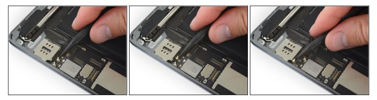
• Disconnect the left and right Wi-Fi antenna cables by lifting them straight up from their sockets on the lower end of the logic board.
