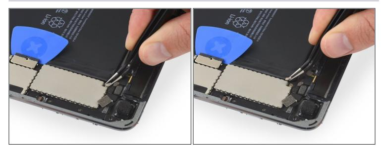
• Disconnect the antenna interconnect cable by lifting it straight up from its socket on the logic board.
