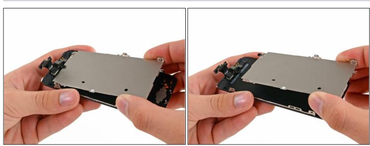
• Remove the LCD shield plate from the display assembly.
