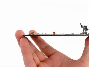
• Remove two 1.2 mm Phillips screws from each side of the LCD frame (four total).
