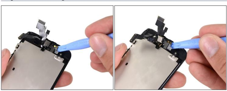
• Starting under the earpiece speaker contacts, use a plastic opening tool or the tip of a spudger to pry the front facing camera cable out of the display assembly.
