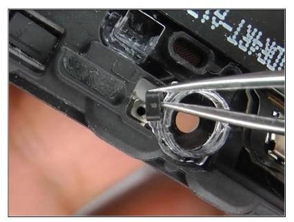
There is a small, black plastic spacer underneath the metal bracket at the upper screw.
