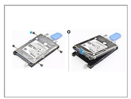
• Remove the screws that secure the hard drive. Lift the hard drive away from the bracket.
