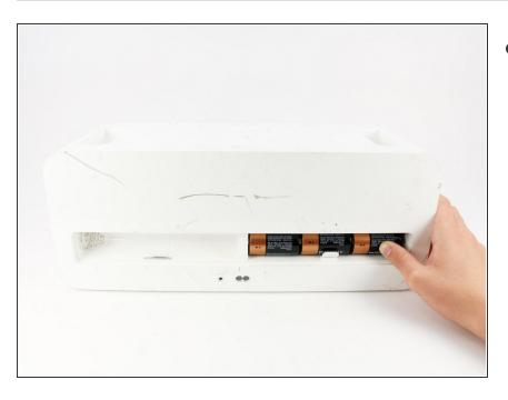
Remove the six D batteries from the device.
