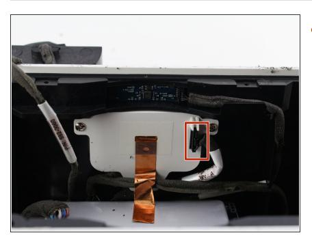
Remove the cable connected to the dock insert by pulling the cable straight out.
