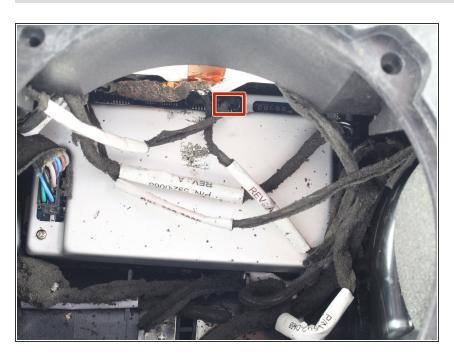
Remove the sensor connection by pulling it straight out with your hand.
