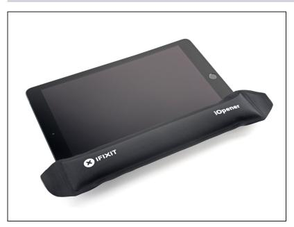
• <u>Heat an iOpener</u> and apply it to the left edge of the device for two minutes.
