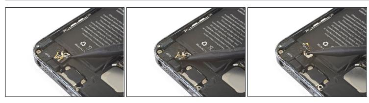
• Slide the point of a spudger underneath the spring contact flex cable below the battery and gently loosen it from the speaker enclosure.
