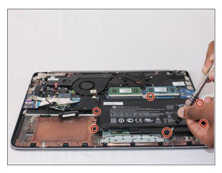
Remove the six 6 mm Phillips #00 screws from the battery.
