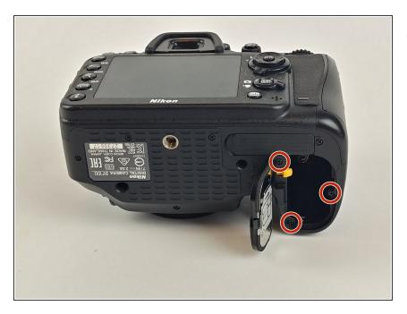
Remove the 3 screws under the battery flap and remove the bottom cover.
