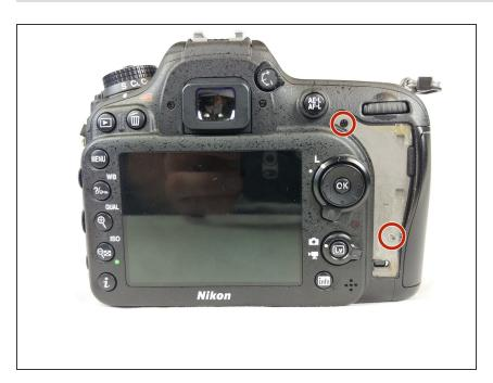
Peel off the adhesive leather screw cover and remove the 2 screws under it.
