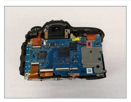
Remove the black 4 pin connector by pulling it out of the connector.
