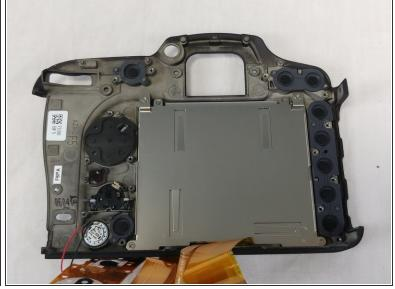
• Unscrew all 16 screws around the back plate of the camera.
