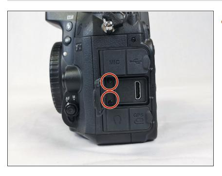
Open the HDMI flap and remove the 2 screws.
