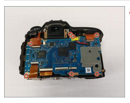
Remove the 7 screws holding the motherboard in place.
