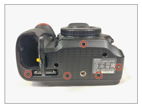
Remove the five screws on the bottom of the camera with a JIS #000 head screwdriver.
