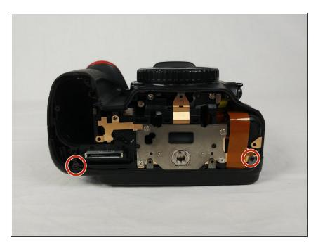
Remove the 2 screws inside the camera on the back corners.
