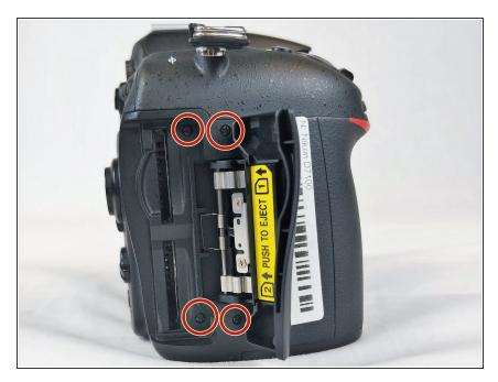
Remove the 2 screws above and below the SD card flap.
