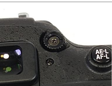
Remove the Diopter adjustment control sticker and remove the screw under it.
