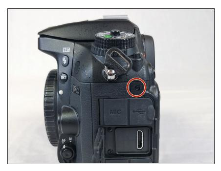
Remove the screw next to the camera strap loop.
