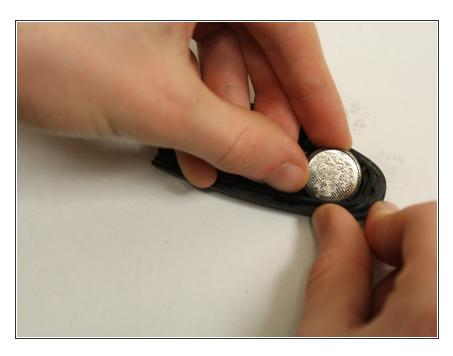
Insert the new battery with "+" facing downward and the "-" facing upward.
