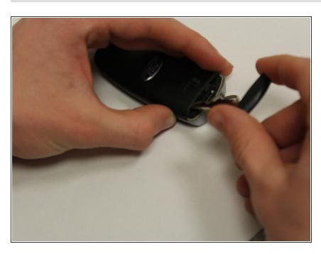
Insert the ignition key in the notch on the left with the FORD logo facing upward.
