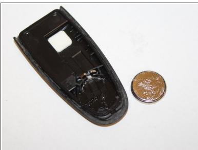
Remove the old battery using the ignition key.
