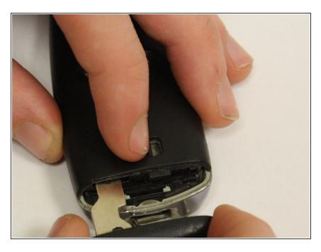
Slide over the key release switch on the back of the fob.
