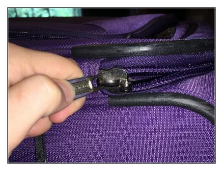
• Applying pressure, use pliers to reattach the metal zipper stopper.
