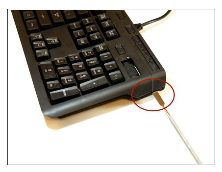
Release the front part using a spudger or flat screwdriver to gently pry. Lift off carefully.
