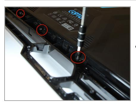
• Flip the keyboard and unscrew the 15 back screws. The screws in the palm rest must be unscrewed and the palm rest removed to access the 6 screws at the bottom of the keyboard. (There are 2 lengths of screws the shorter ones are for the palm rest) There are also 2 screws under the nonslip pads of the palm rest.
