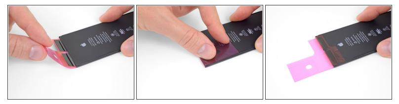
Repeat the previous step to adhere the ends of the two remaining strips at the top edge of the battery.
