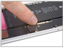
Line up the battery connector and press it into place.
