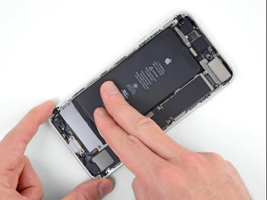
Press the top and bottom areas of the battery firmly into place, allowing the adhesive strips to stick to the rear case.
