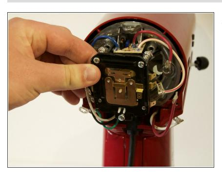
The control plate can now be removed by pulling back on the plate.
