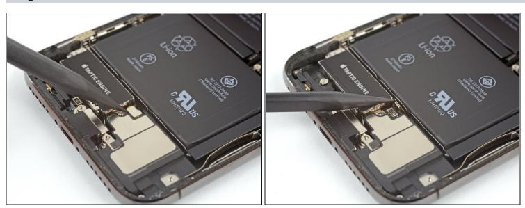
• Use the tip of a spudger to pry up and disconnect the speaker connector.
