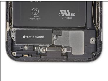
• Remove the 2.1 mm Y000 screw securing the speaker connector cover.
