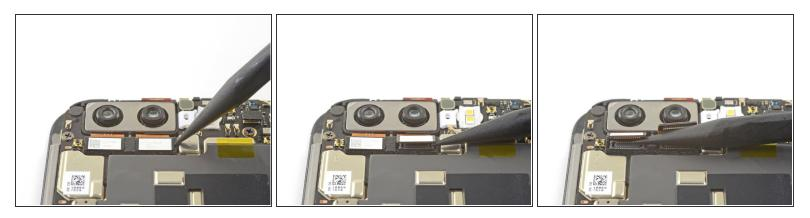
Use the point of a spudger to pry up and disconnect the two rear-facing camera connectors from their sockets on the motherboard.
