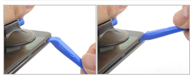
• Lever the opening tool to release the first clip from the frame.
