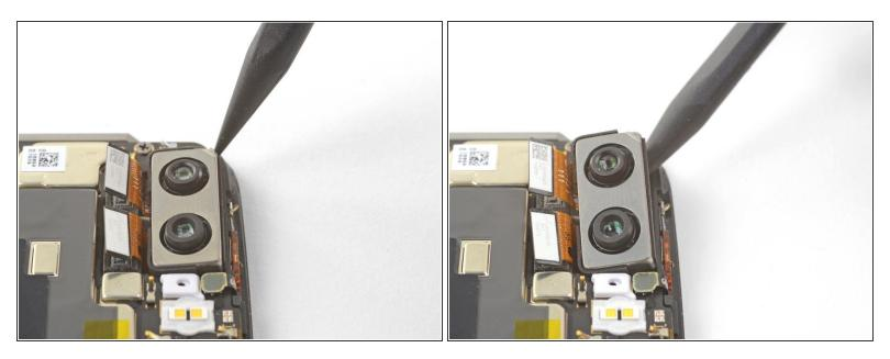
Insert the point of a spudger under the top left corner of the camera module and pry up to loosen it from its recess.
