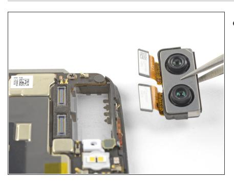
Remove the rear-facing camera module.
