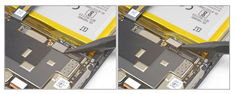
• Use the point of a spudger to pry up and disconnect the battery connector from its socket.
