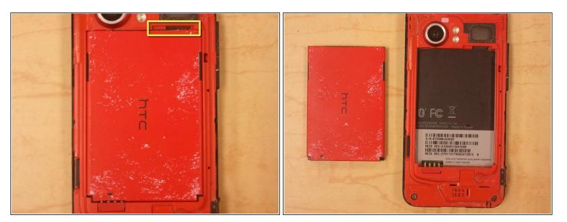
• Remove battery, prying from the provided gap at the upper-right corner of the battery
