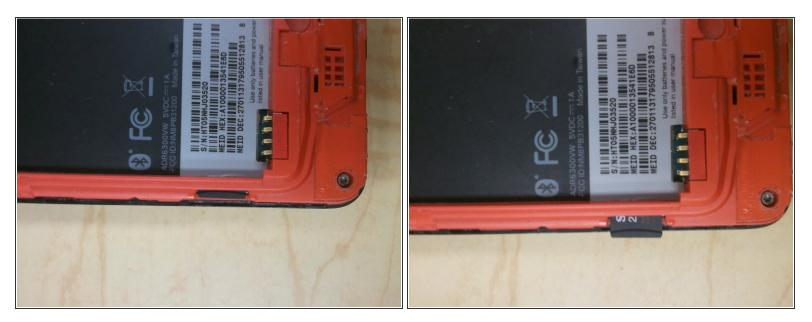
• Depress MicroSD to eject it from the side of the case.
