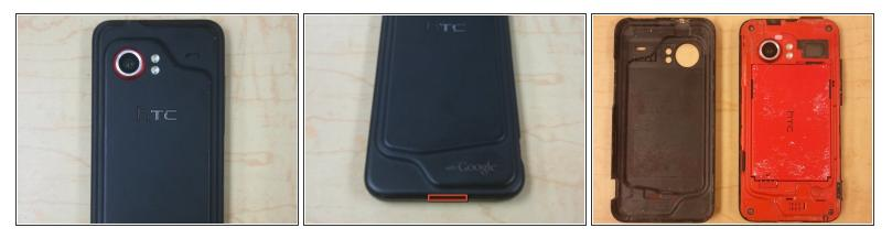
Pry off back plastic, starting at the gap provided at the bottom of the phone. A spudger can be used to make this easier.
