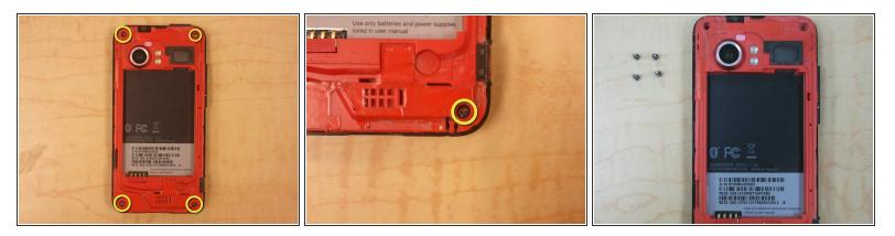
• Remove 4 corner screws, you may have to remove a "VOID" sticker from one of the screw heads.
