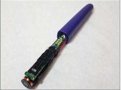
Put the metal head on a solid surface with handle perpendicular to the surface. Firmly, yet gently, push down until the internals start to slide out.
