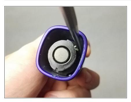
Use a nylon spudger to release the black tabs on either side of internals.
