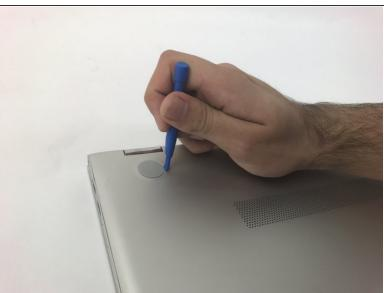
Use the plastic opening tool to remove the gray rubber pads on the bottom of the laptop. For our device we only needed to remove the two at the top.
