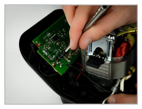
Remove six screws (9mm long, 2mm head diameter) from component housing using Phillips #2 screwdriver
