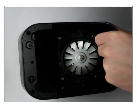
Remove six screws (12mm long, 6mm head diameter) from component housing using Phillips #2 screwdriver.
