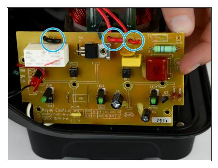
Locate the black and red wire that connect to the circuit. Locate where they are soldered on the back.
