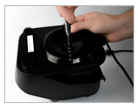
Remove six screws (13mm long, 6mm head diameter) from bottom of the blender using a Phillips #2 screwdriver
