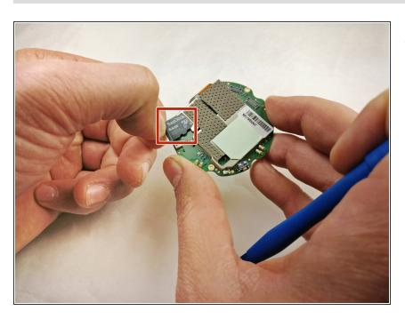
Press and release the SD card to remove it from the circuit assembly.
