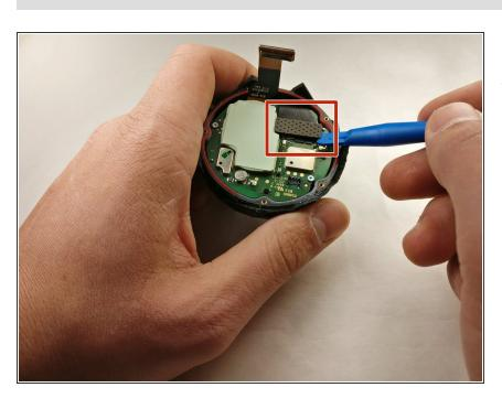
Gently pry the plug from the motherboard and remove the motherboard from the assembly.
