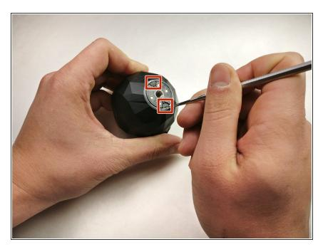
Flip the camera upside down and peel off the two plastic screw covers with the metal spudger to reveal the screws.
