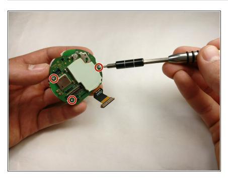
Remove the three 3 mm screws from the circuit assembly with a T4 screwdriver.
