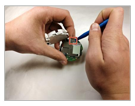
Gently pry out the plug from the circuit assembly.
