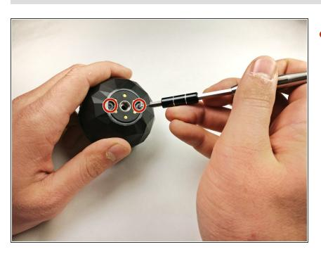
Remove the two 5 mm screws from the bottom of the camera with a T4 screwdriver.
