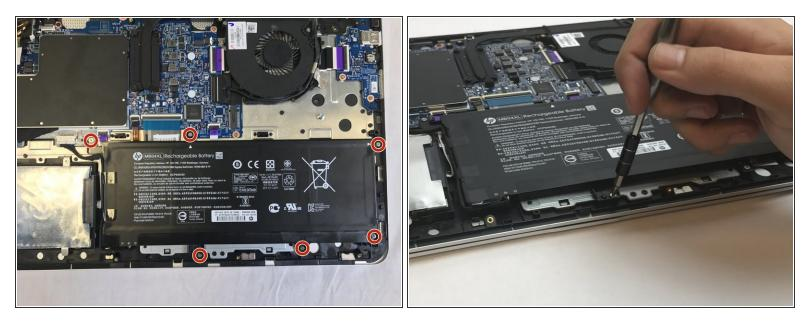
Use a JIS #1 screwdriver to remove the six 4.7 mm screws.
