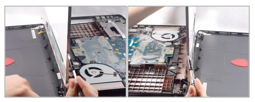
• Unscrew the following screws and remove the screen from the casing.
