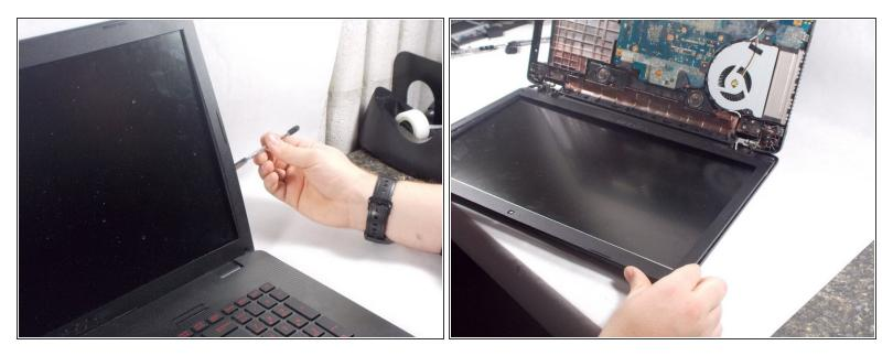
• Use the metal spudger tool to pop out the screen bezel from all four sides.
