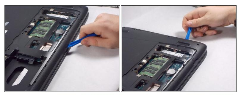
• Use the opening tool to pry the back of the laptop case from the top
