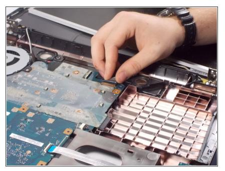
• Remove the SATA cable attached to the screen.
