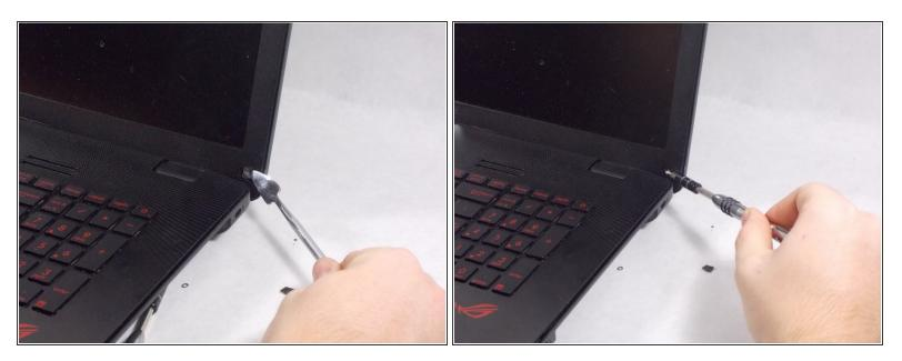
• Remove the two tape covers and screws on the screen bezel.
