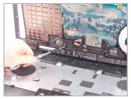
• Unscrew the two 8mm screws attached to the battery
