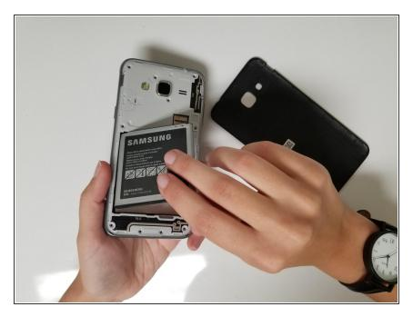
Remove the battery from the casing.
