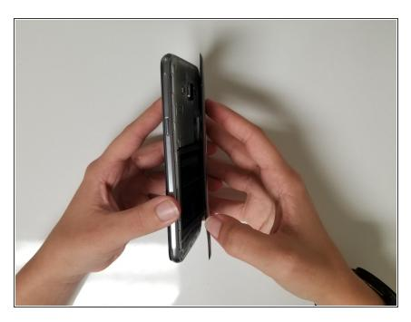
Unplug the device from the charging dock if it is connected. Power off the device. Then using your fingernails, pop off the back cover of the device.
