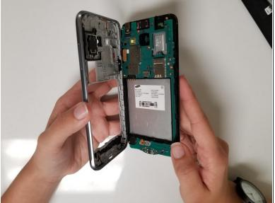
Using a metal spudger, pry the mid frame out.
