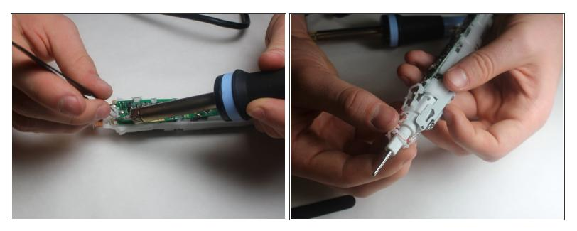
• Use a pair of tweezers to remove the plastic housing and the LED from the device.
