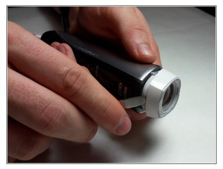
Remove the end cap from the bottom of the toothbrush by prying it off with a spudger.
