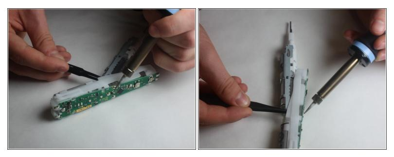
• Desolder the motor terminals from the motherboard and remove the motor assembly.
