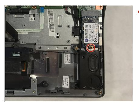
Remove one 6mm screw using a Phillips #0 screwdriver.
