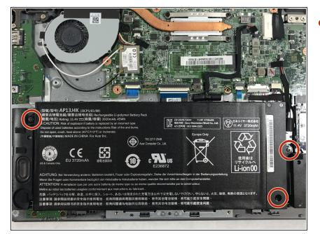
Remove the three 6mm screws indicated by the red circles with a Phillips #0 screwdriver.
