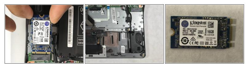
• Carefully remove the solid state drive from the solid state drive slot by sliding it downward away from the motherboard.
